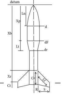
The centers of pressure of nose cones and body transition section are located by dividing the volume of the component by the area at the component's highest datum. This gives the center of pressure location from the component's base. A transform is required to calculate the datum of the CP.
