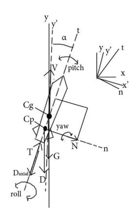
A stable rocket will continuously try to correct its course and return to  $\alpha$  = zero. However, if the  $\alpha$  increases too much, the Cp will move upwards and could meet or overtake the Cg, which will negate the corrective motions entirely, and make the rocket unstable.
